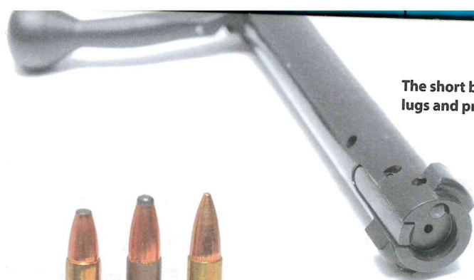
All three cartridges have 55gr bullets. Note the difference in the cartridge overall length.
