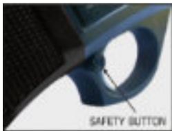
Figure 1a – "ON (SAFE) position"
